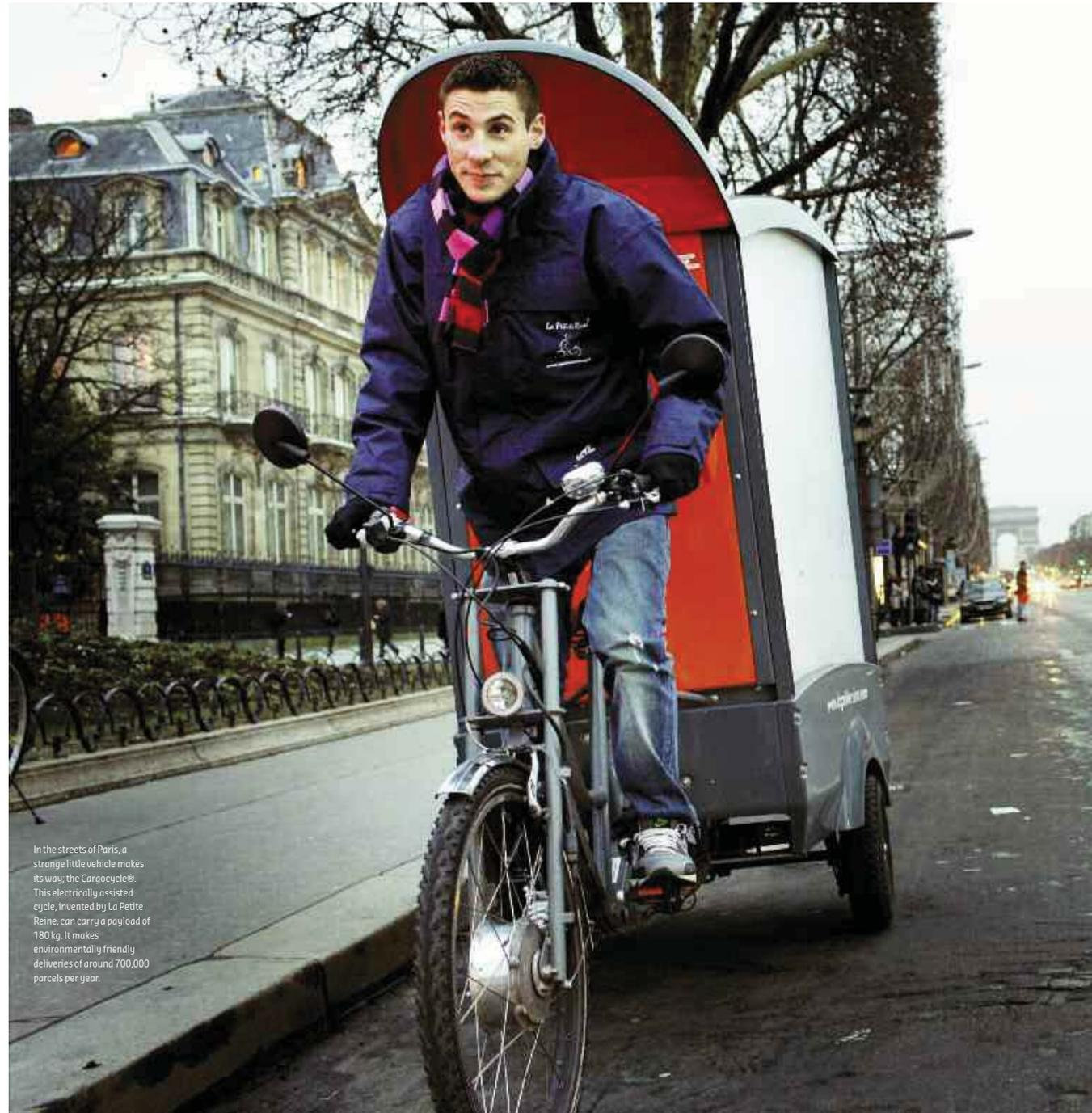
In the streets of Paris, a strange little vehicle makes its way: the Cargocycle®. This electrically assisted cycle, invented by La Petite Reine, can carry a payload of 180 kg. It makes environmentally friendly deliveries of around 700,000 parcels per year.
