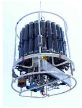
*The instrument platform includes sensors to measure pressure, temperature, salinity, density, chlorophyll, oxygen and turbidity; a volumetric camera to measure animal plankton and marine snow; and bottles programmed to take water samples.*
