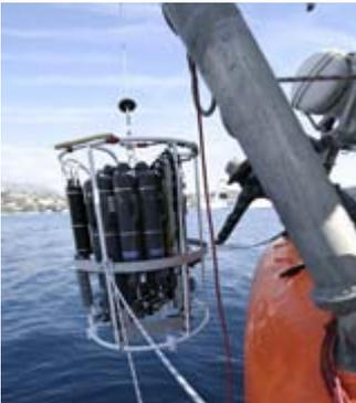
The Veolia Foundation has, in particular, financed the "rose" that was specially designed for the expedition (*see photo opposite*). This apparatus with multiple sensors is able to take samples as well as a wide range of measurements: water turbidity, depth, and so on.
