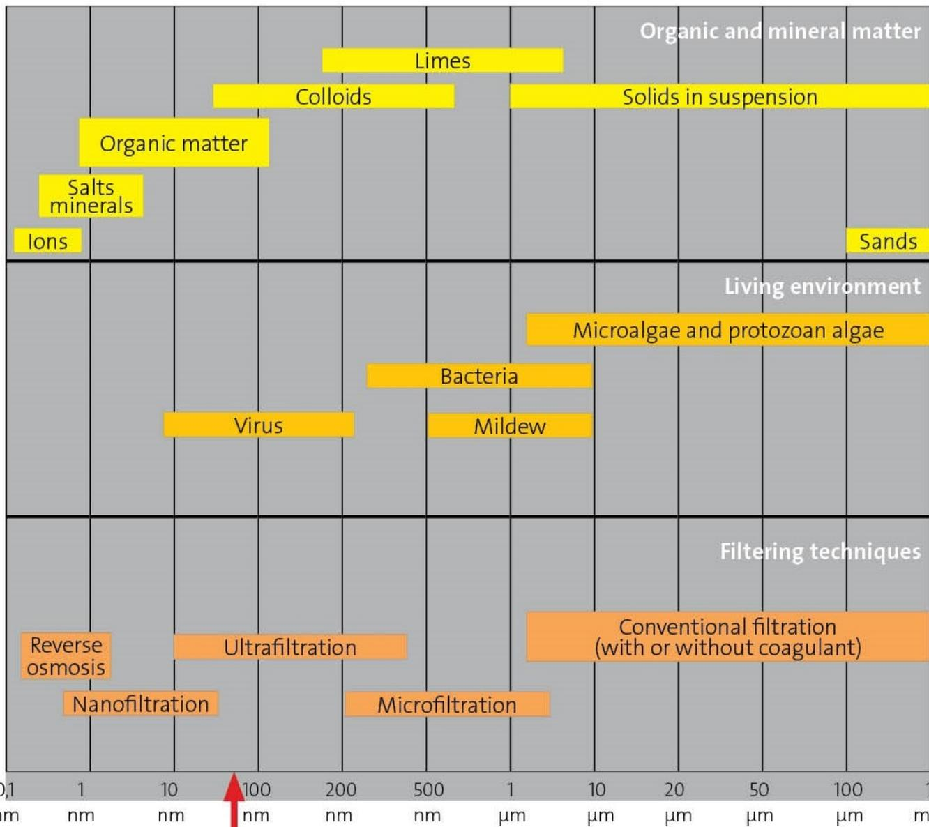
0,1 nm    1 nm    10 nm    100 nm    200 nm    500 nm    1 µm    10 µm    20 µm    50 µm    100 µm    1 mm
